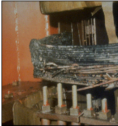
Generator step-up transformer damaged by March 1989 solar storm.
