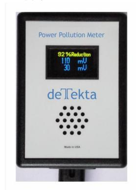
The display screen on the meter above shows the average level of DE (EMI) on a circuit near an outlet before a dirty electricity filter is installed. In this case 110mV. The Meter also shows the new level of local DE (EMI) after installation of filter/s. In this case 30mV, as well as the total percentage reduction achieved in DE levels by filtration. In this case total DE (EMI) levels are reduced by 92% through the use of DE Filters
